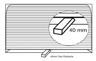
Repeat the test until the safety reverse system works correctly.
