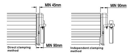
Ensure that there is at least 45 mm from the edge of the curtain to the edge of the bracket. If the roller door drum is on the edge of the curtain or is a smaller diameter, additional clearance may be required.
